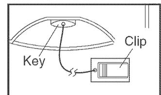
Next, insert the key fully into the console. After a moment, the displays will light. **Test the clip by carefully taking a few steps backward until the key is pulled from the console. If the key is not pulled from the console, adjust the position of the clip.**
