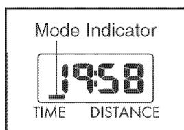
**Calories/Speed display**—This display shows the approximate number of calories you have burned and the speed of the walking belt. The display will change from one number to the other every few seconds, as shown by the mode indicators.
