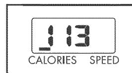
Note: The console can display speed and distance in either miles or kilometers. To change the unit of measurement, hold down the Stop button, insert the key into the console, and continue to hold the Stop button for a moment. An "E" for English miles or an "M" for metric kilometers will appear in the Calories/Speed display. Press the Speed  $\Delta$  button to change the unit of measurement. When the desired unit of measurement is selected, remove the key and then reinsert it.
