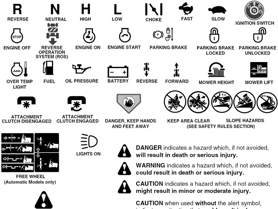
Failure to follow instructions could result in serious injury or death. The safety alert symbol is used to identify safety information about hazards which can result in death, serious injury and/or property damage.
