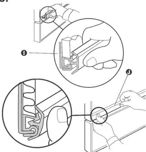
Snap one end of retainer into channel as shown **I**. Push inward while sliding thumb along full length of retainer **I**.
