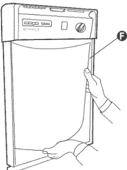
Bow door panel and insert other side of door panel into door frame **F**.
