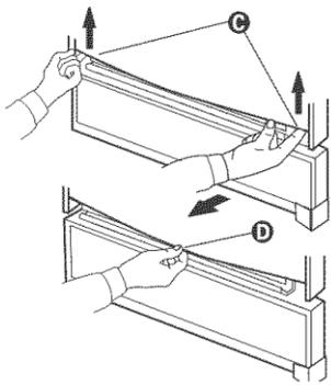
Lift door panel at outer edges **C**. Use one hand to bow bottom of panel **D**. Remove panel. Do not remove spacer.
