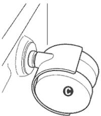
Firmly push casters **C** into holes at corners of dishwasher as shown. Pull on each caster to check that casters are snug.
