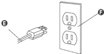
Pull power supply cord **E** from the storage compartment and plug it into the grounded outlet **F**.
