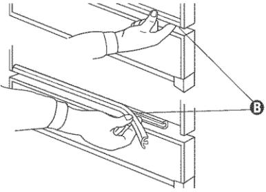
Insert finger under one end of retainer **B** and pull retainer towards you in a peeling action. Set retainer aside.
