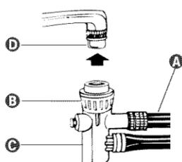
Turn on the hot water faucet until water is hot. Turn faucet off. Pull inlet/drain hose **A** from the storage compartment. Pull down on locking collar **B** and push hose connector **C** over end of faucet adapter **D**. It will snap into place. Release locking collar.
