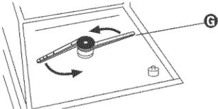
Open dishwasher door and spin the spray arm **G** to check for movement. Close and latch door.
