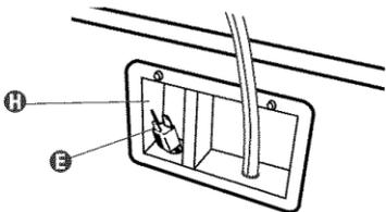
Unplug power supply cord **E** and insert cord into storage compartment **H**.
