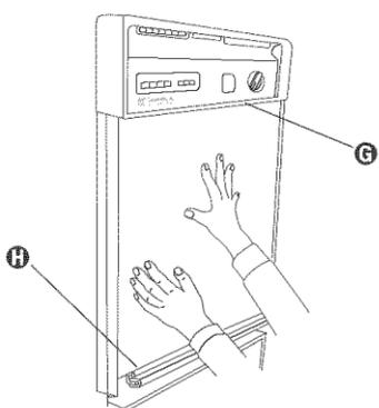
Push in on door panel near the top and slide panel and spacer up inside bottom of control console **G**, allowing panel to rest on channel **H** at bottom of door.
