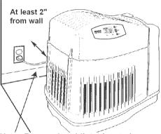
Note: Be sure humidistat located approximately 4 inches outside humidifier body on power cord is free from obstruction and away from any hot air register.
