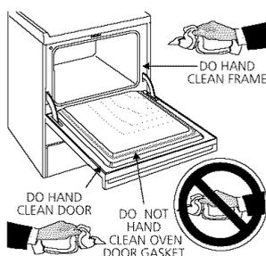
To clean oven door, wash with hot, soapy water and a clean cloth. **DO NOT** immerse the door in water.
