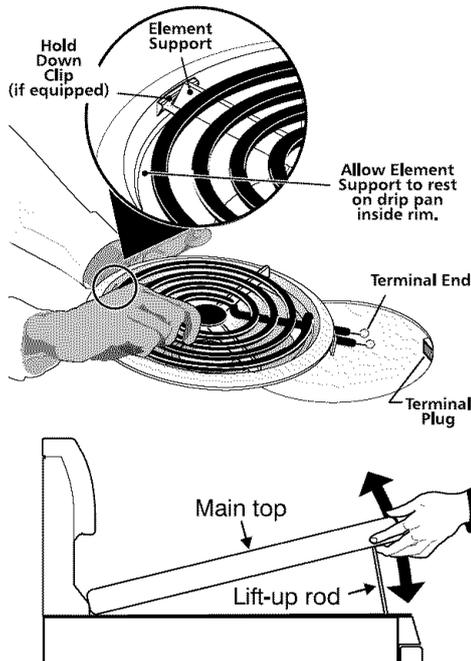
**CAUTION** When lowering the lift-up range top, grasp the sides with finger-tips only. Be careful not to pinch fingers. **DO NOT** drop or bend the range top when raising or lowering. This could damage the surface.
