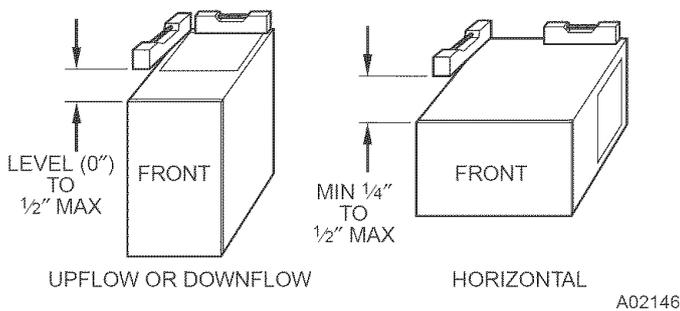
**Fig. 13—Proper Condensate Drainage**
