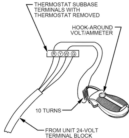
EXAMPLE:  $\frac{5.0 \text{ AMPS ON AMMETER}}{10 \text{ TURNS AROUND JAWS}} = 0.5 \text{ AMPS FOR THERMOSTAT SETTING}$
