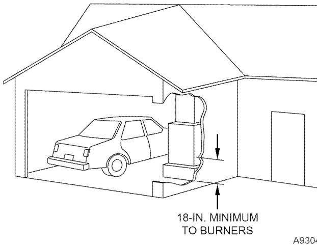
Fig. 16—Installation in a Garage
