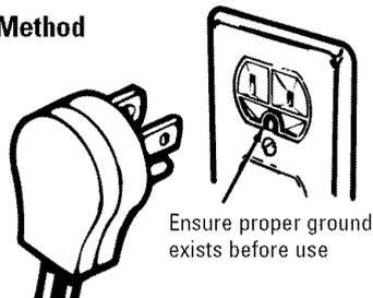
The power cord of this appliance is equipped with a 3-prong (grounding) plug which mates with a standard 3-prong grounding wall receptacle to minimize the possibility of electric shock hazard from this appliance.
