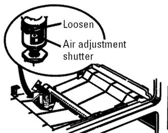
The shutter for the bottom (oven) burner is near the back wall behind the storage drawer or warming drawer. Remove the drawer. See the *Care and cleaning of the range* section.
