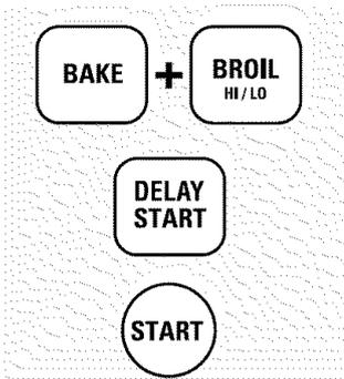
With this feature, should you forget and leave the oven on, the control will automatically turn off the oven after 12 hours during baking functions or after 3 hours during a broil function.
