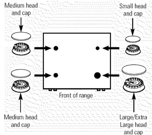
Make sure the slot in the burner head is positioned over the electrode.
