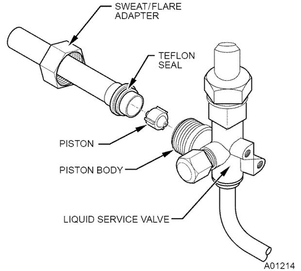
**Fig. 8—Liquid Service Valve with Sweat Adapter Tube**
