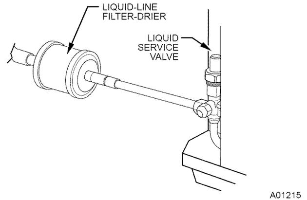
**Fig. 9—Filter Drier with Sweat Adapter Tube and Liquid Tube**
