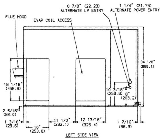
**REQ'D CLEARANCES FOR SERVICING, in. (mm)**
