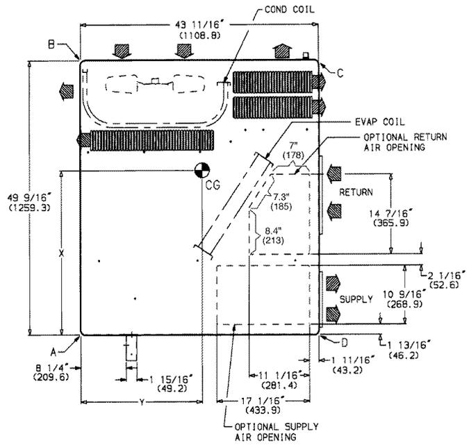
**REQ'D CLEARANCES FOR SERVICING. in. (mm)**
