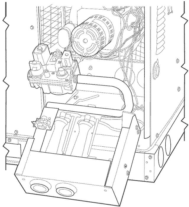
Fig. 27 — Burner Rack Removed
