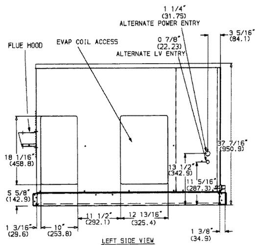
**REQ'D CLEARANCES FOR SERVICING, in. (mm)**
