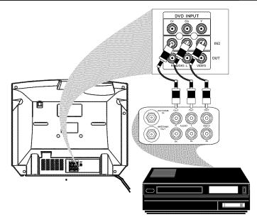
There are AUDIO and VIDEO IN1 jacks at the lower-right corner of the rear of the TV set. To view material playing on equipment connected here, press the TV/AV so AV1 is shown on the TV.
