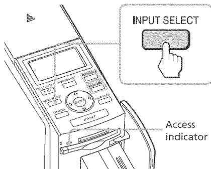
The access indicator flashes and the images are loaded into the printer. The LCD display of the printer shows the current image number.
