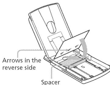
**6** Set the paper tray into the printer and press PRINT. The cleaning cartridge and protective sheet will clean inside the printer. After the cleaning is finished, the protective sheet is automatically ejected.
