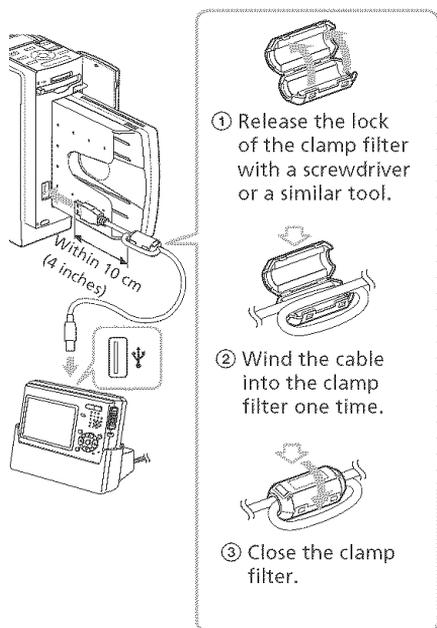
Attach the clamp filter as close to the plug as possible (within 10 cm (4 inches)) that is connected to the printer's USB connector.
