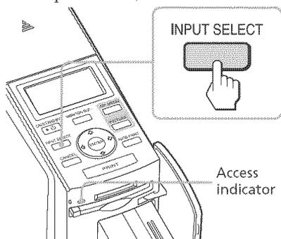
The access indicator flashes, and the images on the selected memory card are displayed on the TV monitor. This is called the **image list**.
