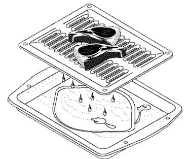
The broiler pan and the insert (if equipped) allows grease to drain and be kept away from the high heat of the broiler. **DO NOT** use the pan without the insert. **DO NOT** cover the insert with foil; the exposed grease could ignite.
