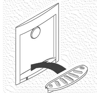
The drip tray for your refrigerator's water dispenser comes from the factory detached. Its removal also allows easy cleaning. To install the drip tray, fit it into the bottom of the dispenser bay and snap into place.
