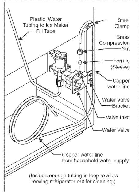
**IMPORTANT:** It takes approximately 24 hours for the ice maker to begin producing usable ice. Air in new plumbing lines may cause ice maker to cycle two or three times before making a full tray of ice. New plumbing may cause ice to be discolored or have poor flavor. Discard ice made during the first 24 hours.
