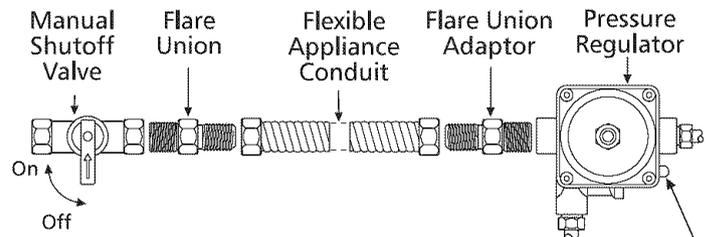
Service Shut-Off Valve Electric Ignition models only
