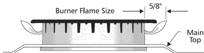
Adjust flame until you can quickly turn knob from LITE to LOWEST POSITION without extinguishing the flame. Flame should be as small as possible without going out.
