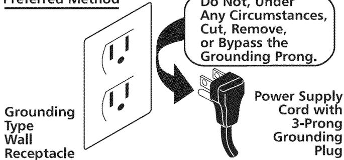
Where a standard two-prong wall receptacle is encountered, it is the personal responsibility and obligation of the customer to have it replaced with a properly grounded three-prong wall receptacle.
