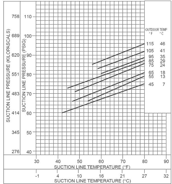
Fig. 23—Cooling Charging Chart, 48GS048 Units <sup>C00047</sup>
