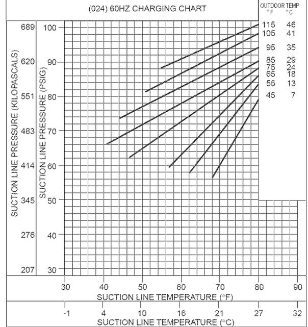
Fig. 25—Cooling Charging Chart, 48GX024 Units <sup>C00049</sup>
