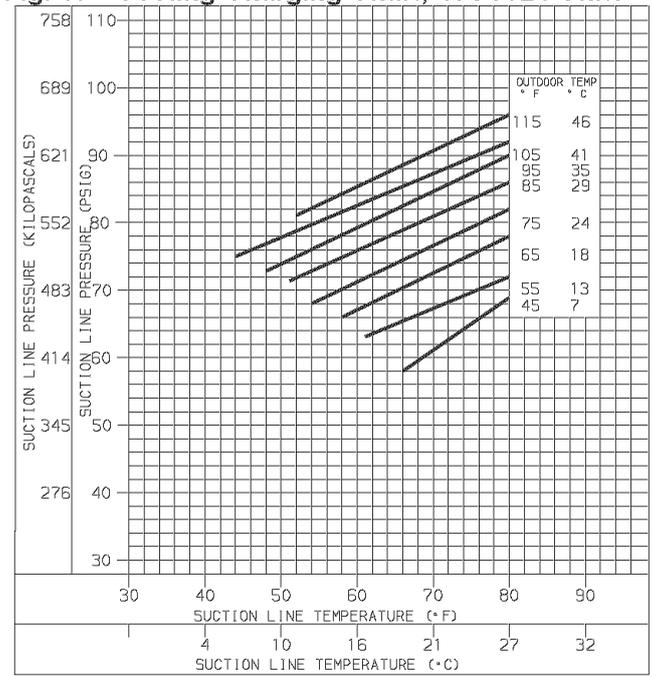
Fig. 21—Cooling Charging Chart, 48GS036 Units C00044
