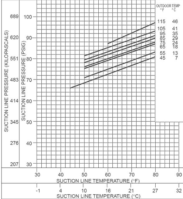
Fig. 24—Cooling Charging Chart, 48GS060 Units <sup>C00048</sup>
