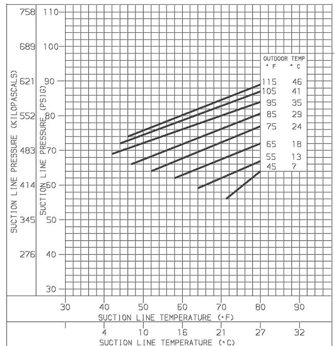
Fig. 19—Cooling Charging Chart, 48GS024 Units C00042
