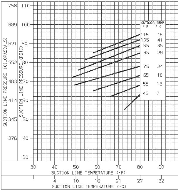
Fig. 22—Cooling Charging Chart, 48GS042 Units <sup>C00045</sup>
