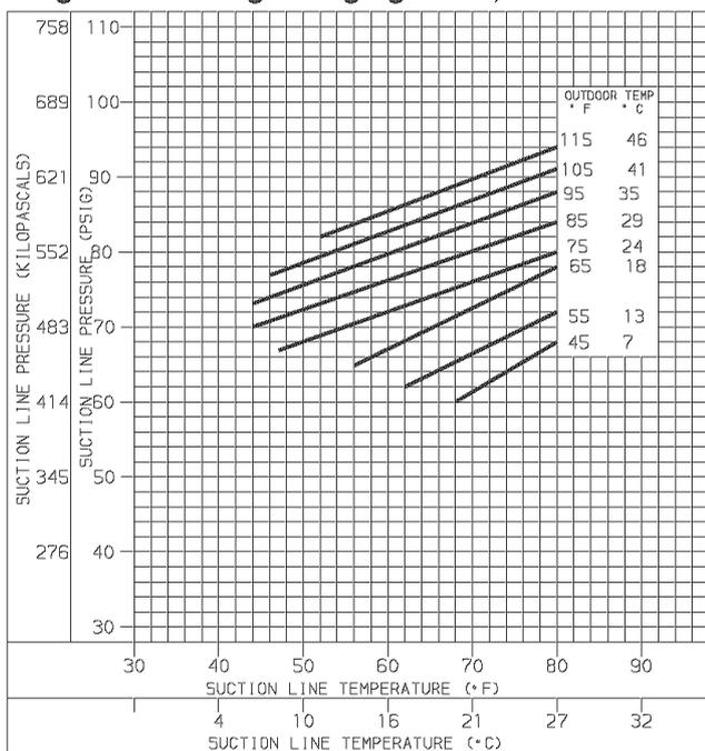
Fig. 20—Cooling Charging Chart, 48GS030 Units C00043
