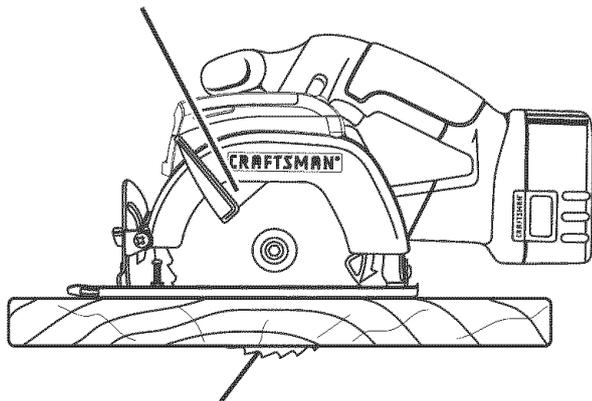
**BLADE EXPOSED ON UNDERSIDE OF WORKPIECE**
