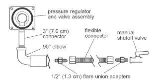
Assemble the flexible connector from the gas supply pipe to the pressure regulator, located in the lower left side of the storage drawer area, in this order: shutoff
