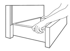
Insert storage drawer into slide rails on sides of drawer opening. Lift front of drawer slightly and push firmly to
