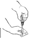
Line up holes in anti-tip bracket with mounting holes in floor. Use the screws provided to fasten anti-tip bracket to floor.
