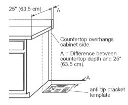
If countertop is not flush to the side of the cabinet opening, align the left side of the template to allow for the countertop overhang. Tape the freestanding range anti-tip bracket template in place.
