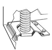
Carefully move range into final position. Look under range (a flashlight may be needed) to check that left rear leveling leg is engaged in the anti-tip bracket. If leveling leg is not properly engaged, remove and reposition the anti-tip bracket to ensure that the leveling leg fits properly in the anti-tip bracket.
