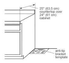
Place the anti-tip bracket template on the floor in the cabinet opening so that the left edge is against cabinet and the top edge is against the rear wall, molding or cabinet. If countertop is deeper than 25 inches (63.5 cm), measure and mark a distance 25 inches (63.5 cm) in from front of countertop opening and align template with mark (or subtract 25 inches (63.5 cm) from the countertop depth and add the difference to the corresponding dimension).
