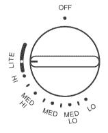
If burners do not light properly, turn cooktop control knob to the "OFF" position. Check that the power supply cord is plugged in and the circuit breaker or fuse has not blown. Check that the gas shutoff valves are set to the "OPEN" position. Repeat Step 22. If a burner does not light at this point, contact your KitchenAid dealer or authorized service company for assistance.
