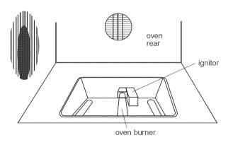
Check the oven burner for proper flame. This flame should have a 1/2" (1.3 cm) long inner cone of bluish-green, with an outer mantle of dark blue, and should be clean and soft in character. No yellow tips, blowing or lifting of flame should occur.
