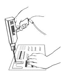
To mount anti-tip bracket to wood floor, use the anti-tip bracket template to mark where to drill mounting holes. Use a drill with a 1/8" (0.3 cm) drill bit to drill the two mounting holes. Remove template from floor.
