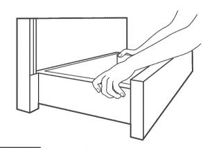
Press on front of storage drawer and release to open. Pull open to first stop position. Lift front of drawer to clear white wheels in drawer guides. Remove drawer and set it aside on a protected surface.
