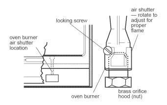
If the oven flame needs to be adjusted, locate the air shutter near the center rear of range. Loosen the locking screw and rotate the air shutter until the proper flame appears. Tighten locking screw.
