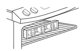
Place rack in oven. Place level on rack, first side to side; then front to back. If the range is not level, pull range forward until the rear leveling leg is removed from the anti-tip bracket. Adjust the leveling legs up or down. Then slide range back into position. Check
