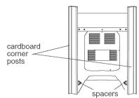
Take 4 cardboard corner posts from the carton. Stack one cardboard corner post on top of another. Repeat with the other two corner posts. Place corner posts lengthwise on the floor in back of range so corner posts will support outer side edges of range as shown.
