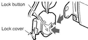
Return the lock cover to the closed position after pulling out the grip belt.
