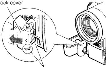
Open the lock cover while pinching the protection portion of both ends.
