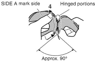
**2** Fit the hinged portion of the other holder piece into the warped hinge portion.
