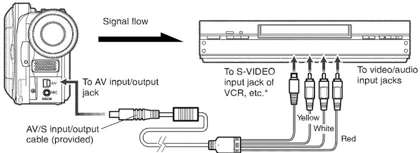
\* If the video device to be connected has an S-VIDEO input jack, you can connect it to the DVD Video Camera.
