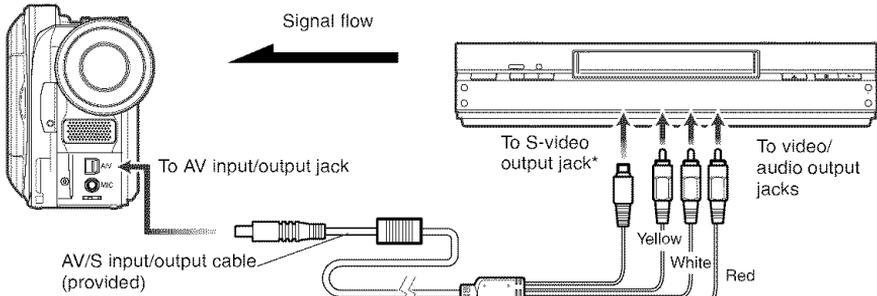
\* If you are using VDR-M70PP and the connected AV device has an S-VIDEO output jack, you can connect the S-VIDEO jack of AV/S input/output cable.
