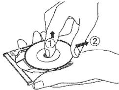
Slide the disc obliquely upward
