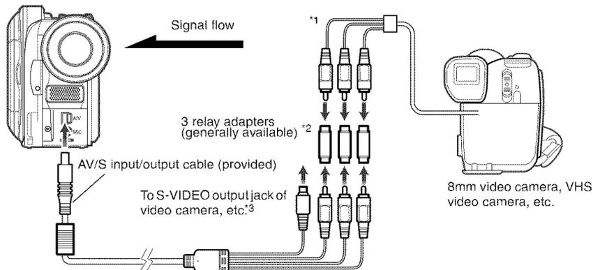
\*1: The AV/S input/output cable provided with this DVD Video Camera can be directly connected to some video cameras.
