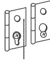
10. Remove door strike plug (B). Insert the door strike you removed in Step 8 in hole and secure with screw. Insert door strike plug in original door strike hole and secure with screw.
