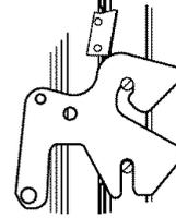
4. Insert the door stop clip with the angular surface at the top of the frame hinge slot, then push in the bottom of the clip until flanges are flush with the front frame.
