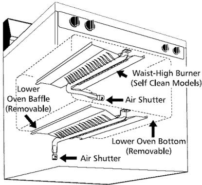
To remove the oven bottom, remove oven hold down screws at rear of oven bottom. Pull up at rear, disengage front of oven bottom from oven front frame, and pull the oven bottom out of the oven. Remove burner baffle so that the burner flame can be observed.
