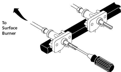
Test to verify if "LOW" setting should be adjusted
