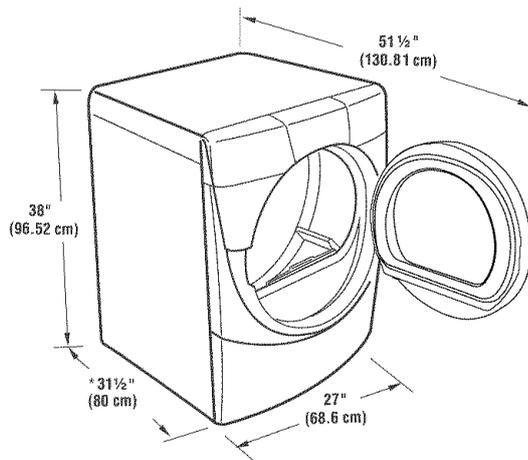
\*Most installations require a minimum 5½ in. (14 cm) clearance behind the dryer for the exhaust vent with elbow. See "Venting Requirements."
