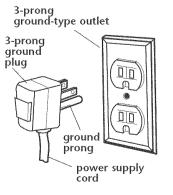
For your personal safety, this washer must be grounded. This washer is equipped with a power supply cord having a 3-prong ground plug.
