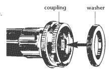
Insert a flat washer into each end of the inlet hoses. Check that washers are firmly seated in couplings.
