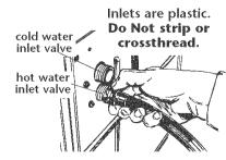
Attach one hose to the hot Attach one nose to the not water (bottom) inlet valve first; then other hose to the cold water (top) inlet valve. Tighten couplings by hand. Then use pliers to make an additional two-thirds turn.
