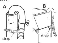
Put "hook" end of drain hose in laundry tub or standpipe. Tightly wrap the shipping strap around the drain hose and laundry tub or standpipe as shown in Figures A-B. Push plug into the nearest hole in the shipping strap.
