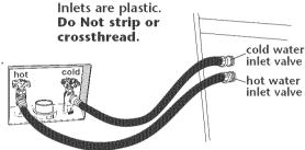
Attach bottom hose from the inlet marked "H" to the hot water faucet. Attach top hose from the inlet marked "C" to the cold water faucet. Tighten couplings to faucets. **DO NOT OVERTIGHTEN**; this could cause damage to couplings.
