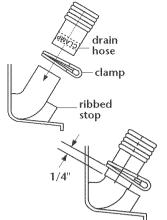
To prevent the drain hose from coming off or leaking, it must be installed per the following instructions.
