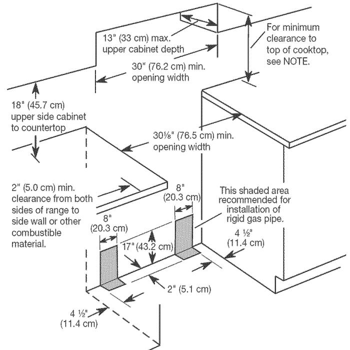
**NOTE:** 24" (61 cm) minimum when bottom of wood or metal cabinet is protected by not less than 1/4" (0.64 cm) flame retardant millboard covered with not less than No. 28 MSG sheet steel, 0.015" (0.4 mm) stainless steel, 0.024" (0.6 mm) aluminum or 0.020" (0.5 mm) copper.
