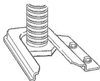
5. If installing the range in a mobile home, you must secure the range to the floor. Any method of securing the range is adequate as long as it conforms to the standards in the "Location Requirements" section.
