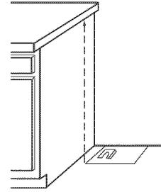
If cabinet opening is wider than specified in the "Location Requirements" section, adjust template so range will be centered in cabinet opening.
