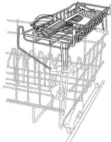
The utensil rack lies on the two supports in the right-hand lower rack. Load the rack tray while it is in the dishwasher or remove it for loading on a counter or table top.
