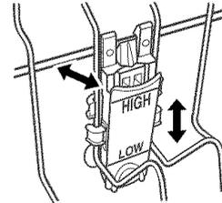
2. With the other hand, pull out the top of the adjuster.
