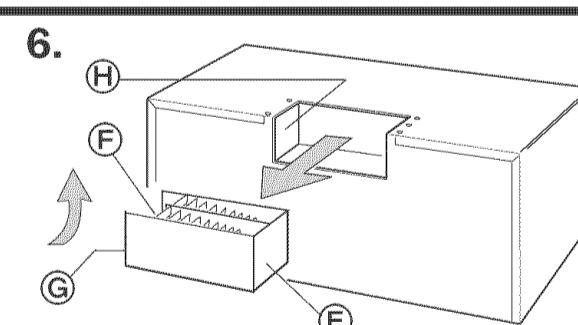
Slide air deflector back into cabinet as far as it will go. Check that deflector vanes **F** face the top of the cabinet and that the small exhaust ports **G** **H** face each other.
