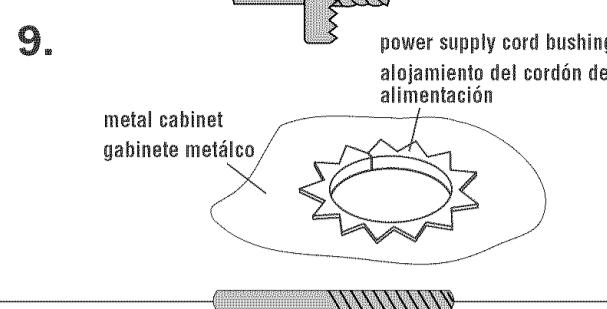
Drill 3/8" holes at points "J" and "K" on upper cabinet template. These are for 2, 1/4-20 x 3" round head bolts and washers used to secure microwave hood to upper cabinet.
