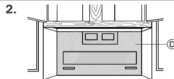
Finger tighten the toggle bolts **A** to make sure toggle nuts **C** have opened against drywall **E**.
