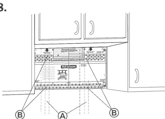
Use a hole drill or key hole saw to cut a 2" diameter hole at shaded area marked "M" on upper cabinet template.
