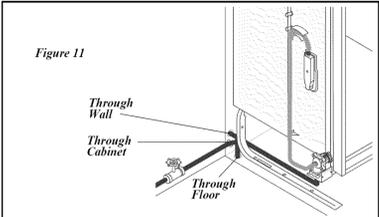
2. Route water line to water inlet valve as shown in **Figure 11**.
