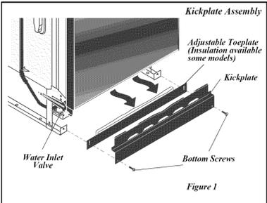
3. Locate water inlet valve behind kickplate on bottom left underside of unit. The valve has a  $\frac{1}{2}$ " NPT female fitting.
