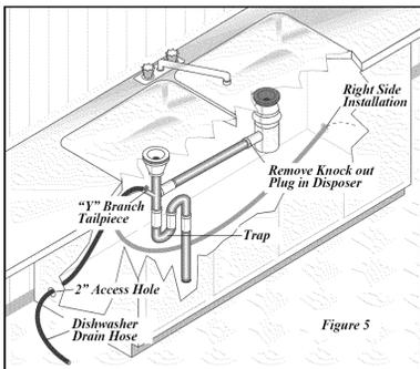
2. If you connect to a sink drain, entry will need to be above trap. A "Y" branch tailpiece and connector kit, not included, will make this method easier and includes all needed fittings and instructions. See **Figure 5**.
