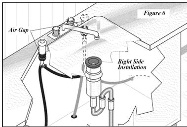
3. If you connect to a sink trap, local codes may require you to install an air gap kit, not included. The drain hose will be routed from dishwasher to air gap inlet as shown in **Figure 6**. An air gap kit is available from a plumbing supply store.
