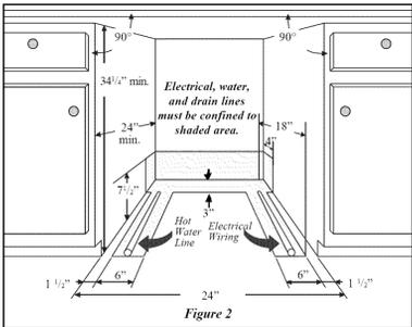
**IMPORTANT:** For proper operation and appearance of unit, cabinet opening should have dimensions as shown in **Figure 2**. If unit is to be placed in a corner, there must be at least a 2-inch side clearance to open door.
