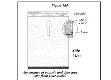
6. Unlatch door and open while supporting outer door on both sides at bottom to keep in place. Align screw holes and replace screws.
