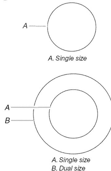
The Dual-Size Elements offer flexibility depending on the size of the cookware. Single size can be used in the same way as a regular element. The dual size combines both the single and outer element and is recommended for larger size cookware, large quantities of food and home canning.
