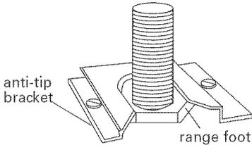
**8.** If installing the range in a mobile home, you must secure the range to the floor. Any method of securing the range is adequate as long as it conforms to the standards in the "Mobile home installation" section.
