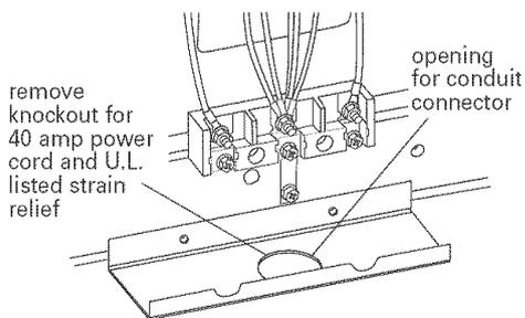
3. Assemble a U.L.-listed strain relief in the opening.
