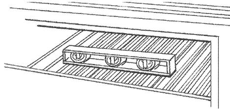
If range is not level, pull range forward until rear leveling leg is removed from the anti-tip bracket. Use 3/8" drive ratchet and channel lock pliers to adjust leveling legs up or down until range is level. Push range back into position. Check that rear leveling leg is engaged in anti-tip bracket.
