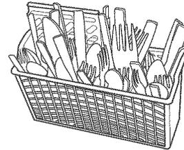
Place small items such as baby bottle caps, jar lids, corncob holders, etc., in the covered section. Close the cover to hold small items in place.
