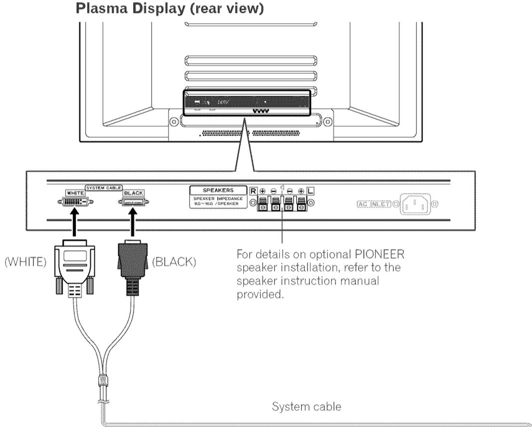
**Connecting the system cable to the Media Receiver**
