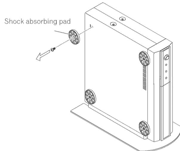
Keep the shock absorbing pads and screws. They are required when you place the Media Receiver in the horizontal position.
