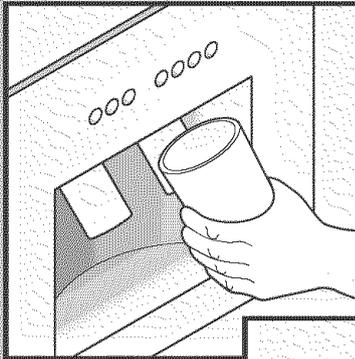
Your automatic ice & water dispenser includes a control panel, a drinking glass bay, and two push-paddles for turning on the ice and water supplies.
