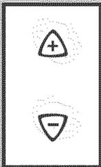
To adjust the temperature to a higher or lower setting, press the **Up** or **Down Arrow** button closest to the display. The first time you press the button, the display shows the last setting you entered. Each press of the button after that increments the setting by one degree.
