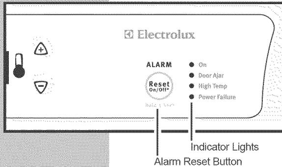
The electronic control system continuously monitors your refrigerator/freezer for temperature consistency, doors left ajar, and power failures. Variances from normal operating conditions are communicated by audible tones and a set of four status indicator lights.
