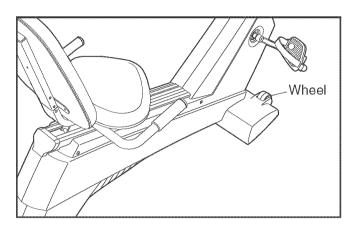
If the exercise cycle rocks slightly during use, turn the leveling feet under the rear stabilizer until the rocking motion is eliminated.
