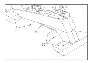
Next, remove the indicated M5 x 25mm Screw (61) and M4 x 16mm Screws (57) from the Right Side Shield (27). Using an adjustable wrench, turn the Right Pedal (21) counterclockwise and remove it. Turn the Right Crank Arm (23) so that it is pointing toward the front of the exercise cycle, and then slide off the Right Side Shield.
