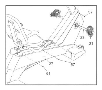
Locate the Reed Switch (46). Turn the Right Crank Arm (23) until the Magnet (30) is aligned with the Reed Switch. Loosen, but do not remove, the indicated M4 x 16mm Screw (57). Slide the Reed Switch slightly closer to or away from the Magnet. Then, retighten the Screw. Turn the Right Crank Arm for a moment. Repeat until the console displays correct feedback. When the Reed Switch is correctly adjusted, reattach the right side shield and the right pedal.
