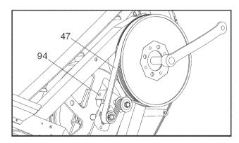
Next, turn the indicated M8 x 35mm Screw (94) until the Drive Belt (47) is properly tightened. Then, reattach the right side shield.
