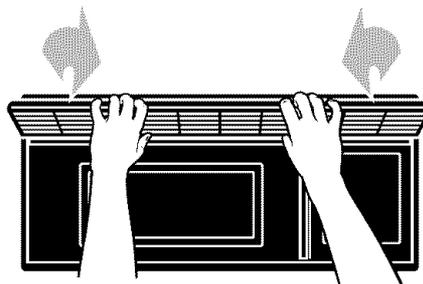
8. Slide the top of the vent grille into place. Push the bottom until it snaps into place. Replace the mounting screws.
