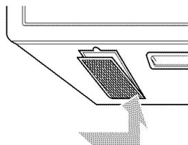
4. To replace grease filters, slide filter in the frame slot on one side of the opening. Push filter upward and push to the other side to lock into place.
