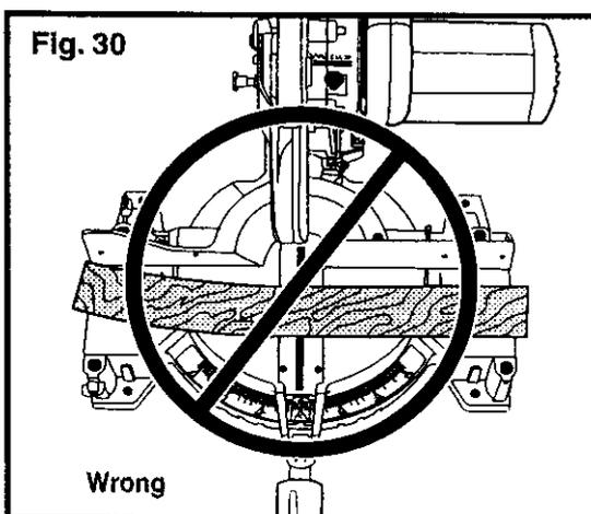
**⚠ WARNING:** To avoid kickback and to avoid serious personal injury **NEVER** position the concave edge of bowed or warped material against the fence.
