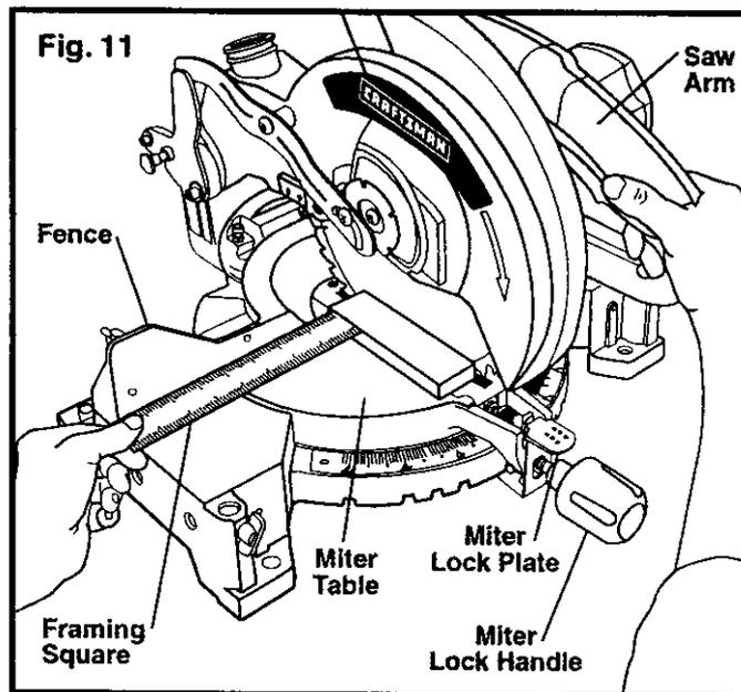
**NOTE:** Be sure that the square contacts the flat side of the blade, not the carbide teeth. This can be easily done by easing the saw arm down with the blade in the throat plate until the carbide teeth are below the table.
