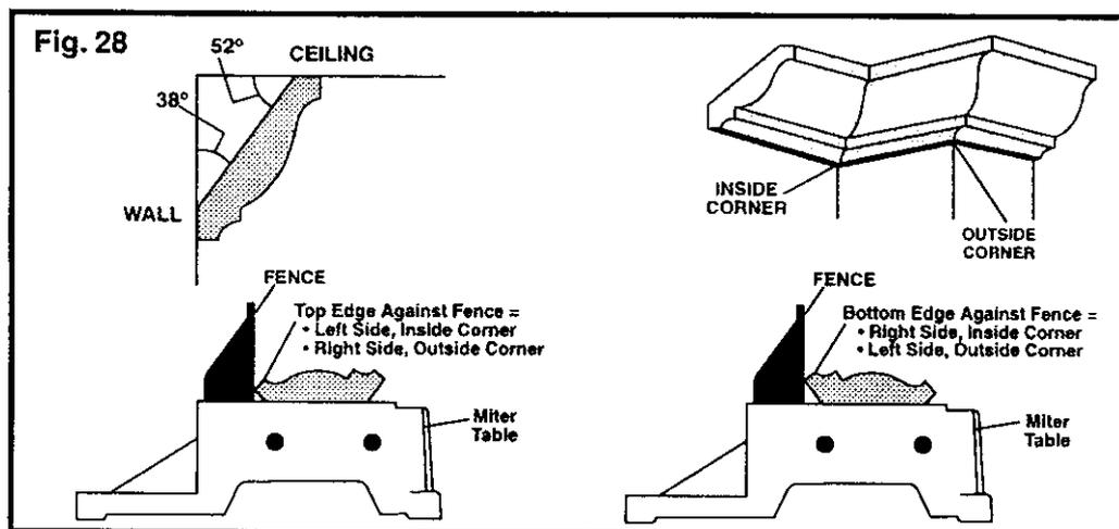
Crown Molding Flat on Miter Table
