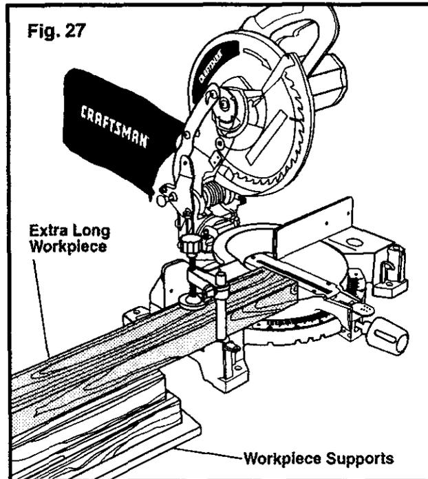
**⚠ WARNING:** To avoid serious personal injury, **ALWAYS** keep your hands outside the "no hands zone" (red lines); at least 3 inches from blade. Also, **NEVER** perform any cutting operation "freehand" (i.e. without holding workpiece against the fence); the blade could grab the workpiece, causing it to slip and twist.
