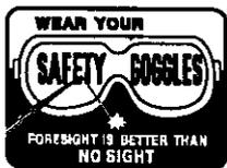
**⚠ WARNING:** The operation of any saw can result in foreign objects being thrown into your eyes, which can result in severe eye damage. Before beginning power tool operation, **ALWAYS** wear safety goggles or safety glasses with side shield and a full face shield when needed. We recommend a Wide Vision Safety Mask for use over eyeglasses or standard safety glasses with side shield, both available at Sears Retail Stores.
