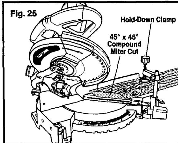
**⚠ WARNING:** To avoid serious personal injury, ALWAYS keep your hands outside the "no hands zone" (red lines); at least 3 inches from blade. Also, NEVER perform any cutting operation "freehand" (i.e. without holding workpiece against the fence); the blade could grab the workpiece, causing it to slip and twist.
