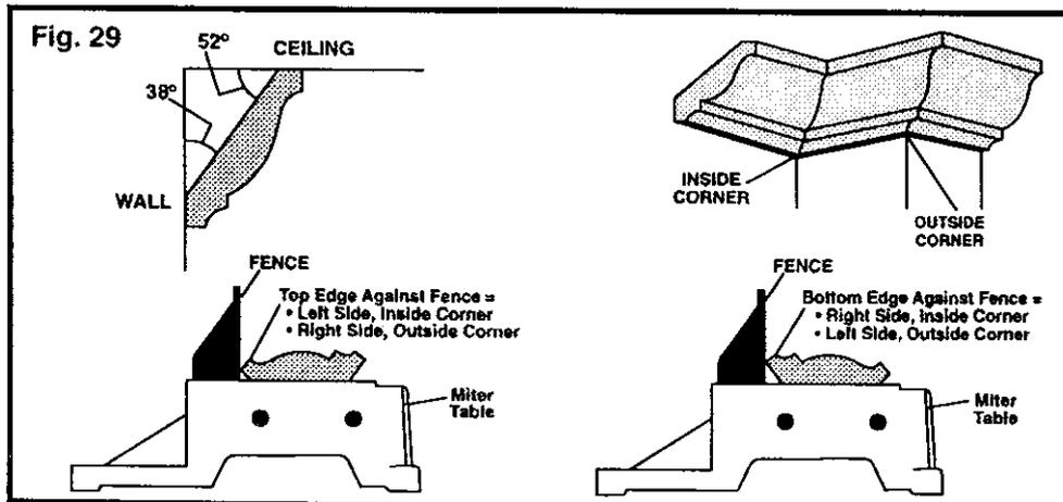
Crown Molding Flat on Miter Table
