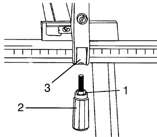
1. Lift upward on rip fence handle (2) so the rear holding clamp is fully extended..
