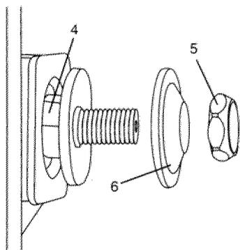
7. To tighten the arbor nut (5) place the open-end wrench jaws on the flats of the saw arbor to keep the arbor from turning. (Fig. J)
