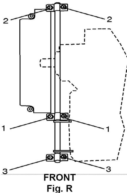
4. While standing at the rear of the saw, use a medium size flat blade screwdriver and gently pry the rear of the blade alignment rod to the LEFT or RIGHT. Using the framing square, simultaneously measure the distance at the front and rear of the blade to an edge of a miter slot. When the distances are within  $1/64$ " or closer, tighten both rear blade alignment rod strap bolts (2) while holding the rod firmly in place.
