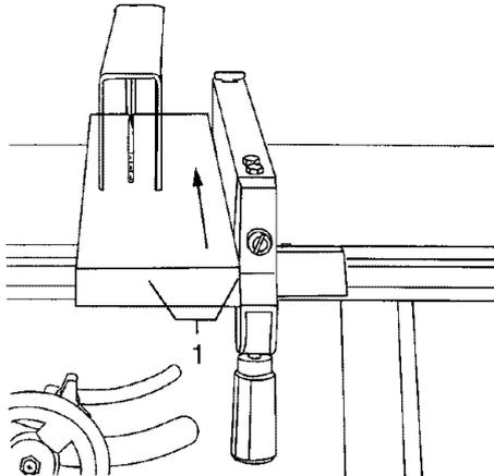
6. Keep your thumbs off the blade top. When your hand reaches the front edge of the table (2), finish the cut with a push stick (3) (Fig. X). You can make a push stick using the pattern on page 23.
