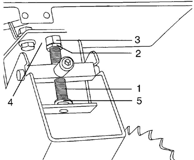
You can place a small amount of dry lubricant on bevel angle adjustment rod also. This rod (1) must be kept clean and free of sawdust, gum, pitch, and other contaminants for smooth operation.
