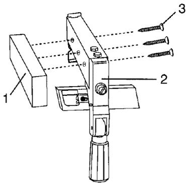
**USING WOOD FACING ON THE RIP FENCE (FIG. DD)**
