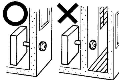
Flue may be positioned directly under opening windows, with a minimum clearance of 9" (230mm).
