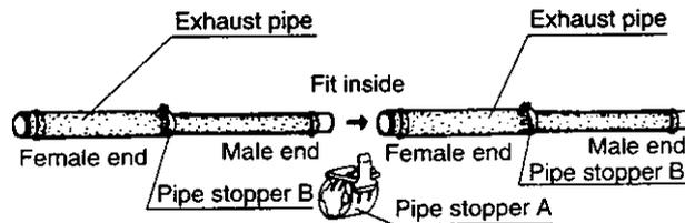
To connect the exhaust pipes, fit the male end into the female end and clamp with pipe stopper A to prevent slipping. The exhaust pipe can be telescoped to the required length; do not cut it.
