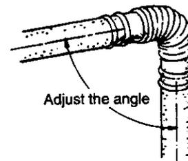
With the exhaust pipes inserted into the ends, bend the bent pipe to the angle required for installation. This part is mainly used for curves and for connection to vent terminal.
