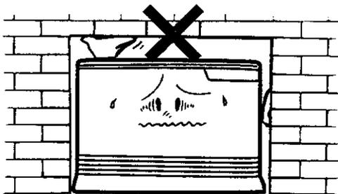
The flue terminal should be positioned away from flammable materials.
