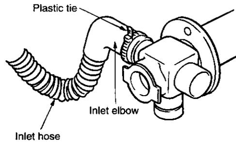
When servicing unit replace plastic tie with new one.
