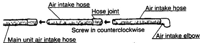
Screw hose joint half of its length onto the air intake hose, then screw another air intake hose into the joint. The hose can be cut to the required length.
