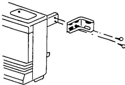
3. Fit Air inlet Hose to heater. Fix Side Back Spacers with screws.
