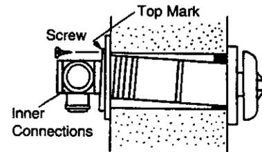
9. Manifold can still be turned after attaching.
