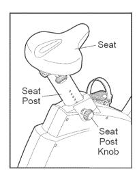
to loosen it (if the knob is not loosened enough, it may scratch the seat post). Next, pull the knob, slide the seat post to the desired height, and then release the knob. Move the seat post up and down slightly until the pin on the knob snaps into one of the holes in the seat post. Then, turn the knob clockwise until it is tight.
