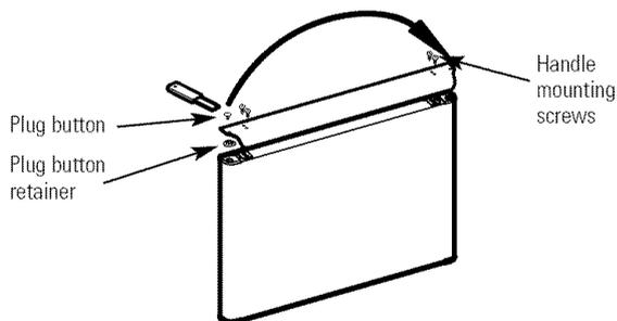
Remove the plug button and transfer it to the opposite side.
