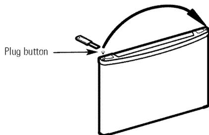
**NOTE:** Make sure the door stop on the bottom of the door has been transferred to the left side of the door as explained in step 6.
