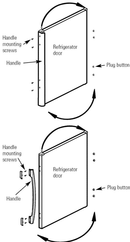
**NOTE:** Make sure the door stop on the bottom of the door has been transferred to the left side of the door as explained in step 6.
