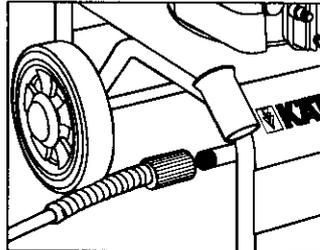
**Step 6** Disconnect the high pressure hose from the high pressure outlet and engage the gun safety lock.
