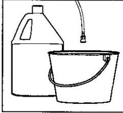
**Step 1** Remove detergent suction tube from container and insert into one gallon of fresh water. Siphon water at low pressure for one minute.
