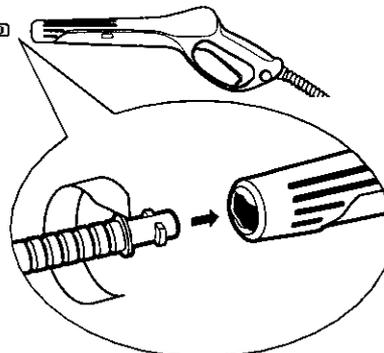
**Step 2** Insert the Vario spray wand into the gun. Push in and turn clockwise to lock spray wand in place.
