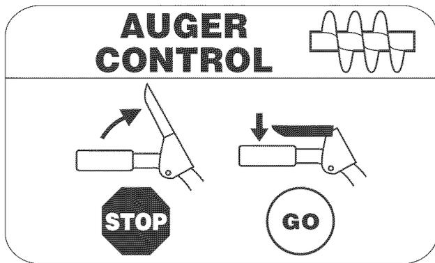
The auger control is located on the **left** handle. Squeeze the control grip against the handle to engage the augers and start snow throwing action. Release to stop.
