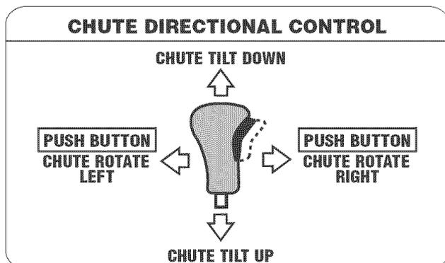
The chute directional control is located on the left side of the dash panel.
