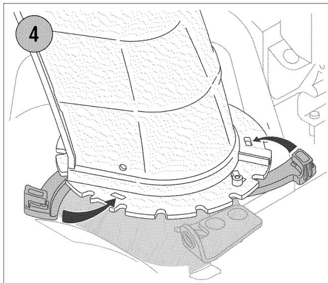
**NOTE:** If the flange keepers will not easily click into place, use the palm of your hand to apply swift, firm pressure to the back of each.
