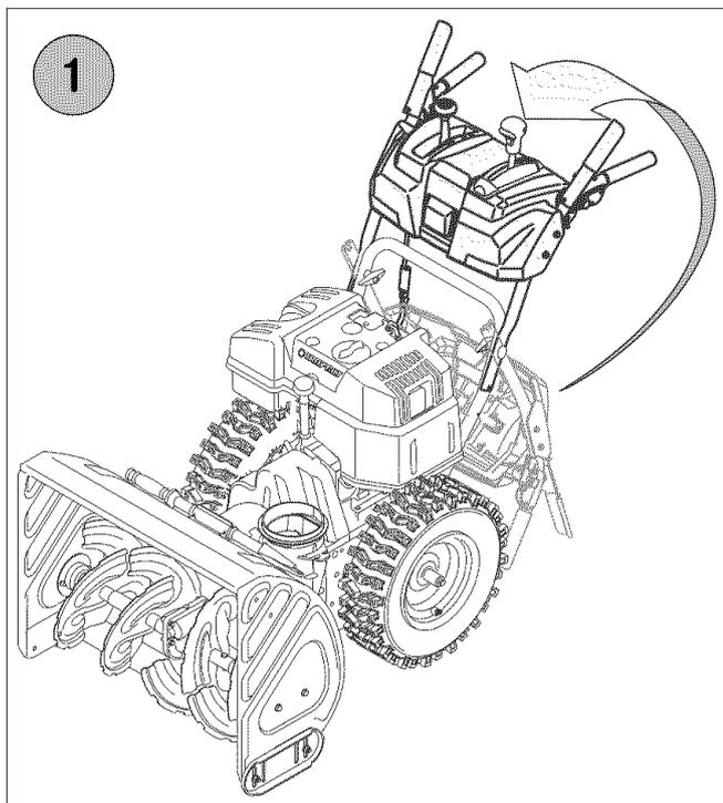
**NOTE:** References to right or left side of the snow thrower are determined from behind the unit in the operating position (standing directly behind the snow thrower, facing the handle panel).
