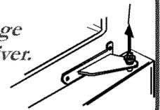
**7** Remove Phillips screws to remove center hinge.
