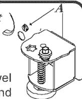
**For Pullout Drawer Models:** After completing the above listed steps, turn roller adjustment screws (A) 2 to 3 times counterclockwise, so that full weight of unit rests on stabilizing legs.
