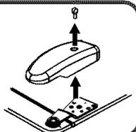
**4** Unscrew 5/16" hex head screws from top hinge to remove hinge.
