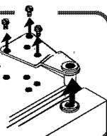
**5** Lift refrigerator door from center hinge pin.
