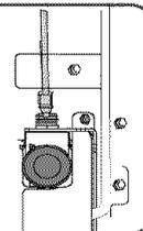
**6** Pull on tubing to confirm connection is secure. Connect tubing to frame with water tubing clamp (F) and turn on water supply. Check for leaks and correct, if present.
