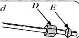
**4** Place end of copper tubing into water valve inlet port. Shape tubing slightly—DO NOT KINK—so that tubing feeds straight into inlet port.
