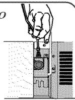
**5** Slide brass nut over sleeve and screw nut into inlet port. Tighten nut with wrench.
