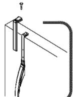
**2** Pry bottom handle trim from handle with screwdriver flat blade wrapped in masking tape.
