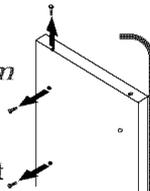
**2** Align handle holes with screw holes on door face and secure with 2 door face screws from step 1.
