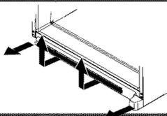
**3** Turn left and right adjustment screws (A) to raise or lower front of refrigerator.
