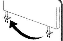
**4** See **How to Install and Remove Handles** to remove and reinstall handles.
