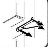
**8** Remove bottom hinge or stabilizing bracket with 3/8" hex head driver.
