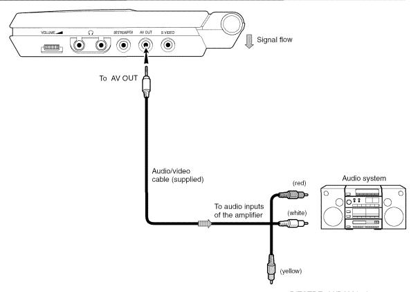
When the AV OUT or BITSTREAM/PCM jacks are connected to the audio input terminals of an audio system, sounds of discs can be heard on the connected audio system. For instructions on connections to audio systems, see also page 57.
