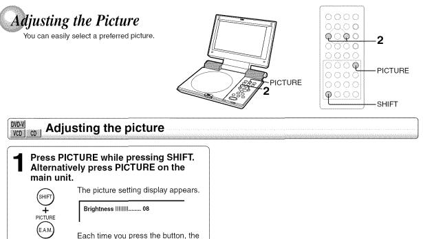
setup items changes as follows. PICTURE Brightness ŧ Color Ŧ Screen ŧ No display Press  $\triangleleft$  /  $\blacktriangleright$  to adjust the value. 2 Brightness: 0 (Darker) to 16 (Brighter) Color : 0 (Paler) to 16 (Deeper) Screen Enhanced : t
