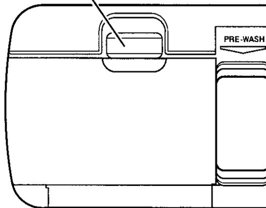
2. Fill the Main Wash section with detergent. The amount of detergent needed depends on the amount of food soil on the dishes and water hardness. See the detergent usage chart on page 13.
