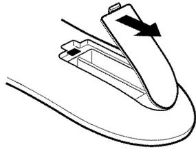
2. Install two "AAA" size batteries. Match the + and - signs on the batteries to the signs on the battery compartment.
