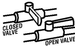
**STEP 4.** Test all the connections by brushing on a soapy water solution (liquid detergent also works well). Bubbles will show a leak. Correct any leak found. Never test for gas leaks with a flame.
