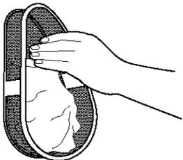
**STEP 4.** Put the lint screen and cover back together and push firmly back into place.
