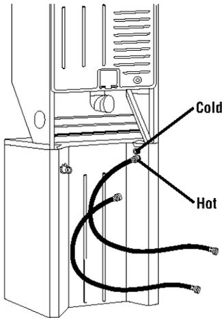
**STEP 3.** Attach the hose with the blue coupling to the cold water (top) inlet valve. Screw on coupling by hand. Make an additional two-thirds turn with pliers to tighten coupling. **DO NOT OVERTIGHTEN;** this could damage valves.
