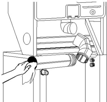
To remove accumulated lint from inside the dryer:
