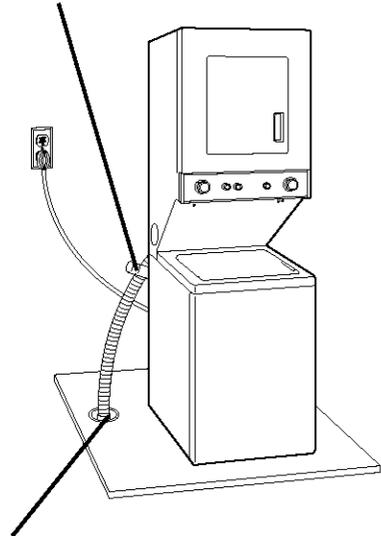
**Floor drain system:** Requires a siphon break, see chart below. A minimum carry-away capacity of 17 gallons per minute is required.
