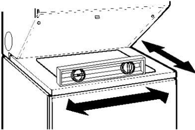
**STEP 2.** If laundry center is not level, prop up the front of the laundry center and adjust the front legs up or down as necessary. Lower laundry center. Repeat STEP 2 until the laundry center is level.
