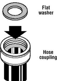
**STEP 2.** Attach the hose with the red coupling to the hot water (bottom) inlet valve. Attaching the red coupling first makes it easier to tighten connection with pliers. Screw on coupling by hand. Make an additional two-thirds turn with pliers to tighten coupling. **DO NOT OVERTIGHTEN;** this could damage the valves.
