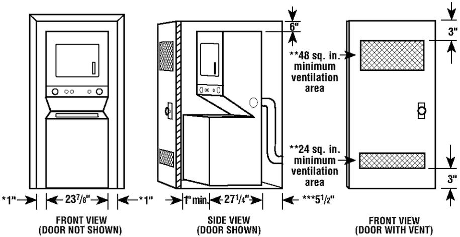
\* Additional clearances for wall, door and floor moldings may be required.
