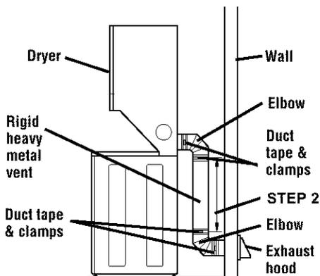
The vent usually comes in 2-foot lengths. Use tin snips to cut the vent 3 inches longer than your measurement in order to make a connection.
