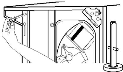
**STEP 3.** Check adjustability of rear legs, by pushing in one leg. The other leg should come out. Check both legs. If they do not adjust, repeat STEP 2.
