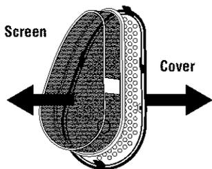
**STEP 3.** Roll lint off the screen with your fingers. Do not rinse or wash screen to remove lint. Wet lint is hard to remove.
