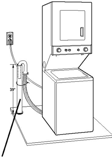
**Standpipe drain system:** Needs a two-inch minimum diameter standpipe with minimum carry-away capacity of 17 gallons per minute. Top of standpipe must be at least 39 inches above floor and no higher than 96 inches from bottom of laundry center.
