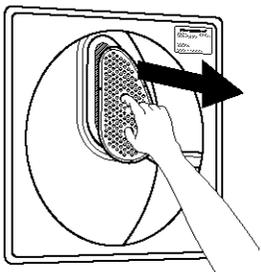
**STEP 2.** Separate the cover and the screen by squeezing the screen and pulling on the cover at the same time.
