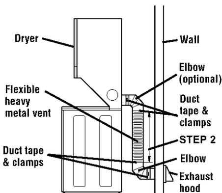
**STEP 3.** Add 10 inches to the measurement for each bend in the vent.
